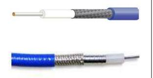
RG 402 (0.141") Semi- Flexible cable offers the best shielding performance with a socked tinned Copper Shielding and Solid Conductor at 0 ~ 18 GHz. It is Commonly equipped with SMA RF Connector for testing adaptor purpose or for high performance device like splitter.
