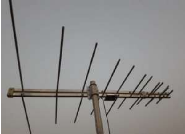
LOG PERIODIC DIPOLE ANTENNA (SRFS 150-500) Frequency: 150~500 MHz / Gain: 12 dBi
